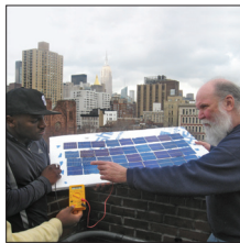
Manhattan Comprehensive students test the wattage of a solar panel they made
